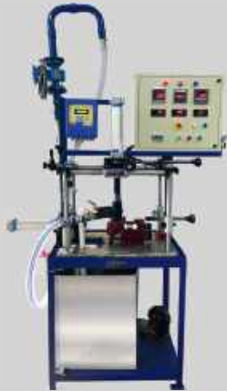
PUMP TESTING MACHINE WITH FLOWMETER & PANEL
