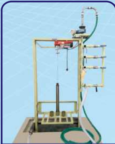
SUBMERSIBLE PUMP TESTING SETUP
